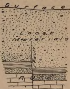
FIG. 60. — Diagram to show how small faults in the rock basement may be masked at the surface through adjustments within the loose rock mantle.
